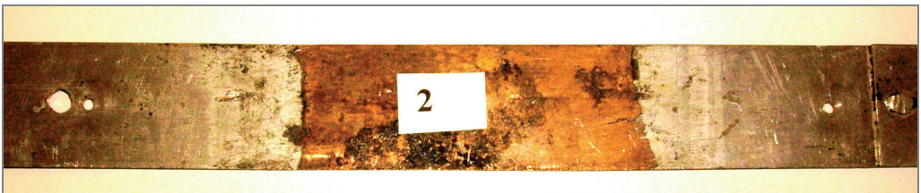
Rys. 2. Fragment chorağiewki wycięty z silnika Fig. 2. Part of the riser cut from the engine
